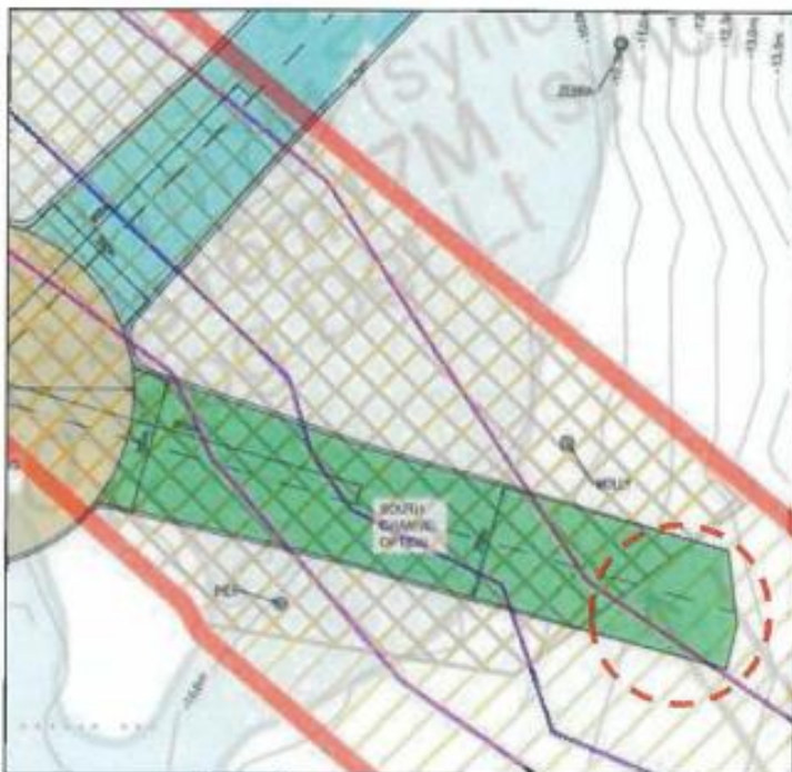
Figure 4 - Area of South approach channel where cable burial appears not to lie within the deeper burial zone
